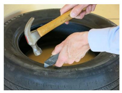
Use a hammer to drive a utility knife blade into the tire, in order to start a cut.
