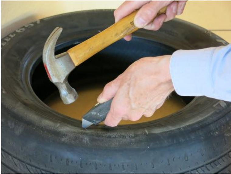
Use a hammer to drive a utility knife blade into the tire, in order to start a cut.
