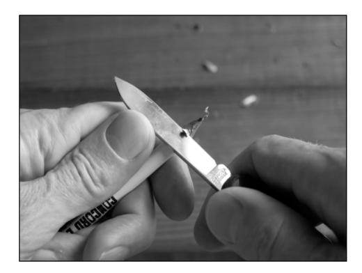
After you have tried whittling a stick for a while, next try to sharpen a pencil with your pocket knife. Again, take SMALL cuts, and always make sure the sharp part of the blade is pointing AWAY from you.
