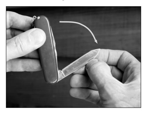
Grasp the blade of the pocket knife with your fingers and your thumbnail, and pull the blade open. (See how there is a little slot in the knife blade where you can put your fingernail?)
