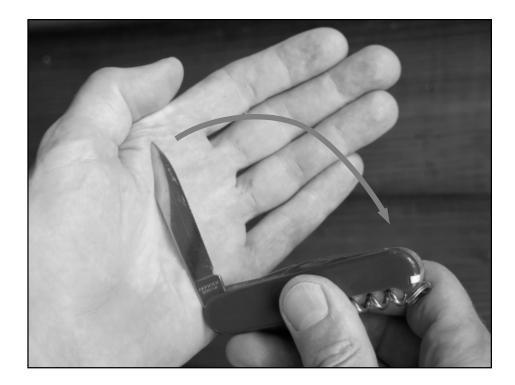
To close a pocket knife, hold the knife in one hand. Make sure your fingers are out of the way of the knife blade.
